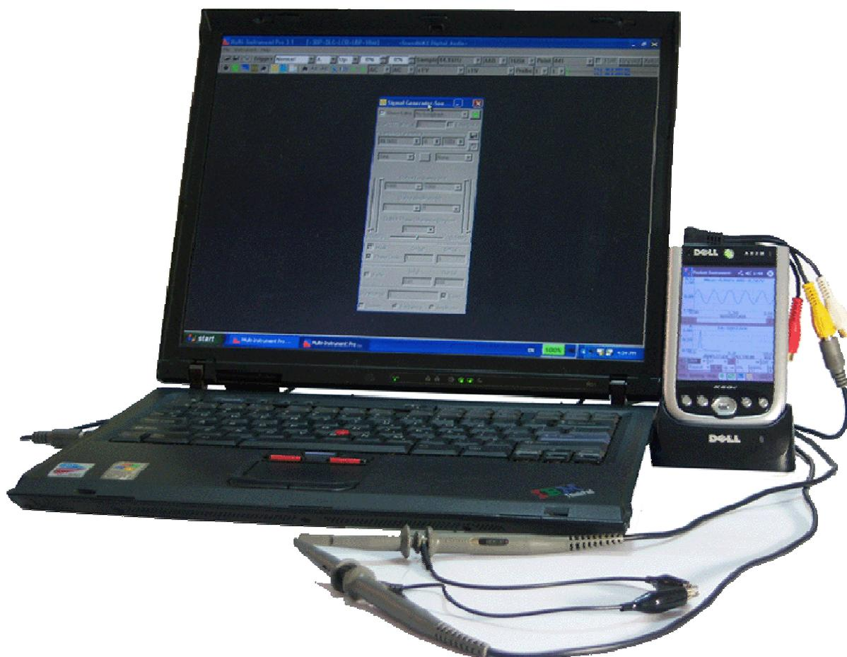
Setup 2 (as shown above) consisted of the same hardware as Setup 1. Unlike Setup 1, in Setup 2, the laptop was used as a signal generator and the Pocket PC was used as an oscilloscope and spectrum analyzer. The connection from the PC to the Pocket PC was made via:
