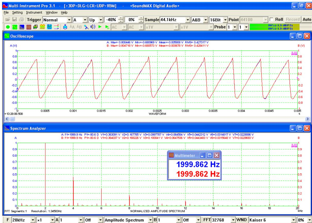
The oscilloscope in the above screenshot shows that the waveform was triggered right at -0.4V (Trigger Level = -40%) upward (Trigger Edge = Up). The sawtooth waveform measured is good in shape.
