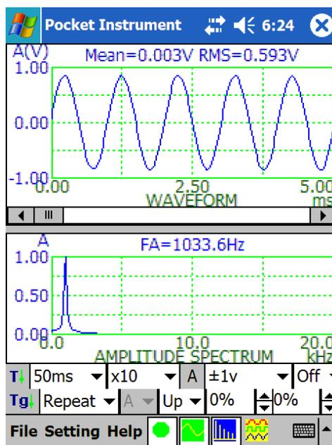
The oscilloscope in the above screenshot shows that the waveform was triggered right at 0V (Trigger Level = 0%) upward (Trigger Edge = Up). The stability of the triggered waveform display was very good. The scan time was set to 50ms. The multiplier of the horizontal axis was set to  $\times 10$  in order to see the individual cycles of the 1kHz sine wave signal. The scan time should be increased if instable triggering occurs.
