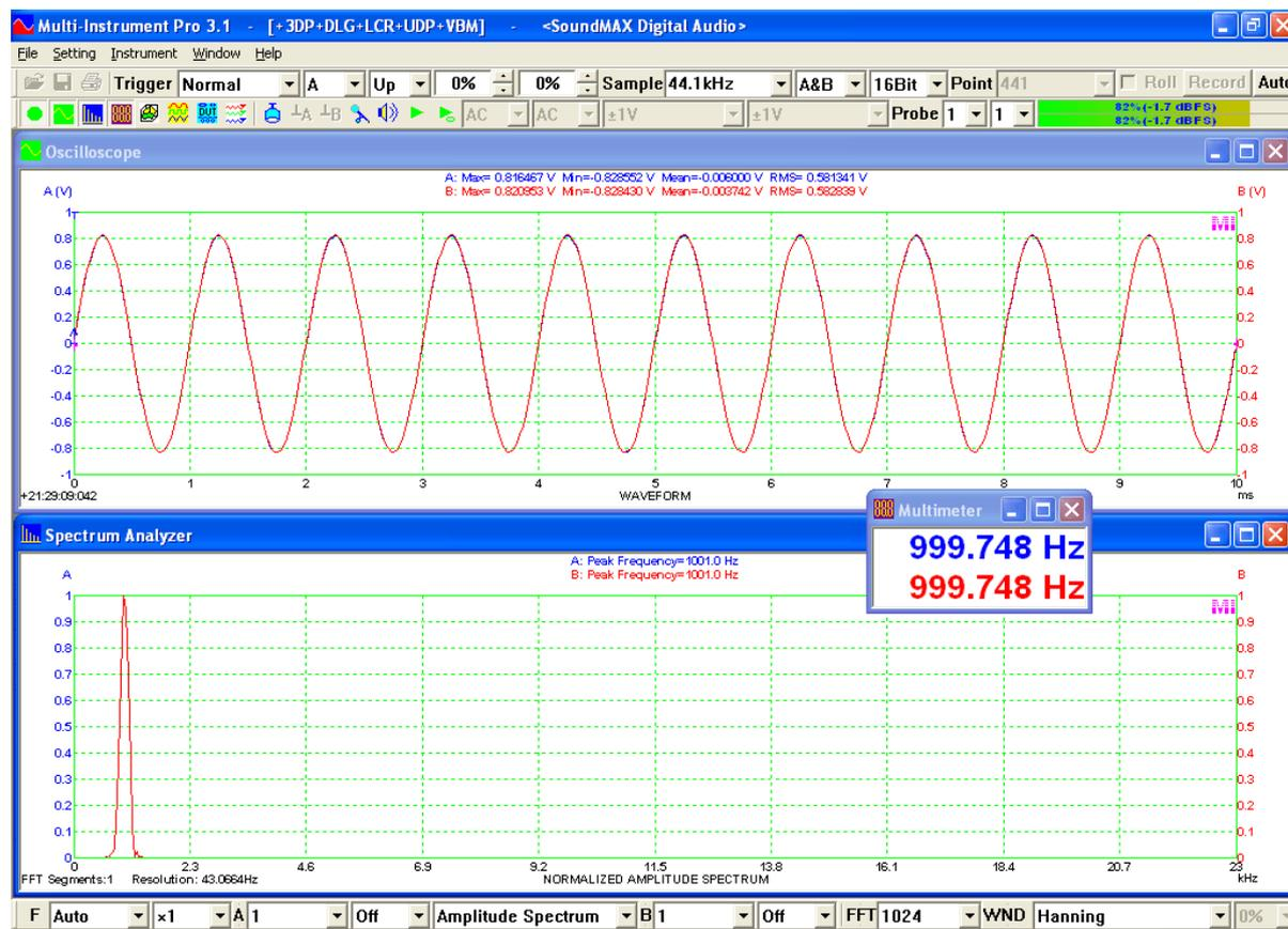
The oscilloscope in the above screenshot shows that the waveform was triggered right at 0V (Trigger Level = 0%) upward (Trigger Edge = Up). The stability of the triggered waveform display was excellent and no shaking left and right or up and down was seen, thanks to the unique algorithm used in the Multi-Instrument software, which is specially designed to overcome the small shaking left and right problem inherent in common software trigger algorithms.
