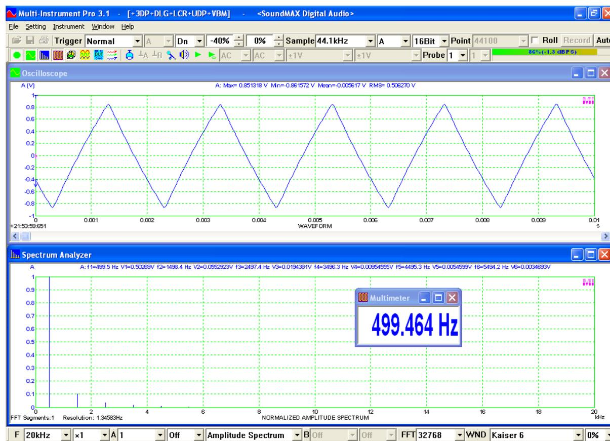
The oscilloscope in the above screenshot shows that the waveform was triggered right at -0.4V (Trigger Level = -40%) downward (Trigger Edge = Down). The triangle waveform measured is very good in shape.
