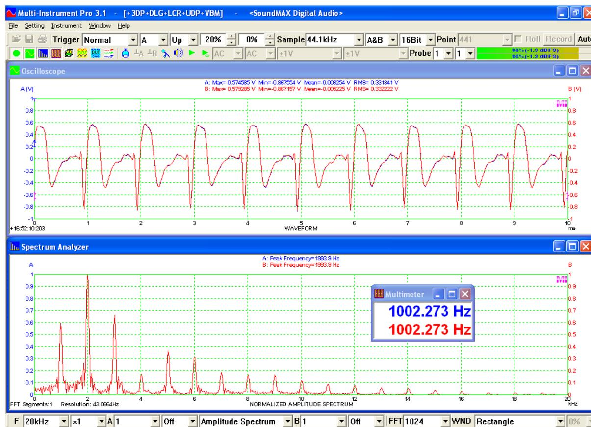
The oscilloscope in the above screenshot shows that the waveform was triggered right at 0.2V (Trigger Level = 20%) upward (Trigger Edge = Up).
