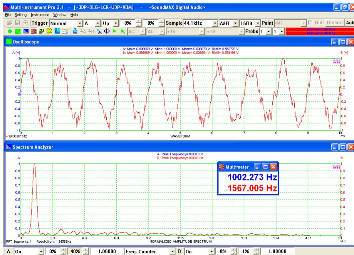
The oscilloscope in the above screenshot shows that the waveform was triggered right at 0V (Trigger Level = 0%) upward (Trigger Edge = Up).
