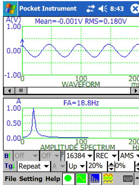
The oscilloscope in the above screenshot shows that the waveform was triggered right at 0.2V (Trigger Level = 20%) upward (Trigger Edge = Up). The stability of the triggered waveform display was very good. The scan time was set to 1s. The multiplier of the horizontal axis was set to  $\times 5$  in order to see the individual cycles of the 20Hz sine wave signal. The scan time should be increased if unstable triggering occurs.
