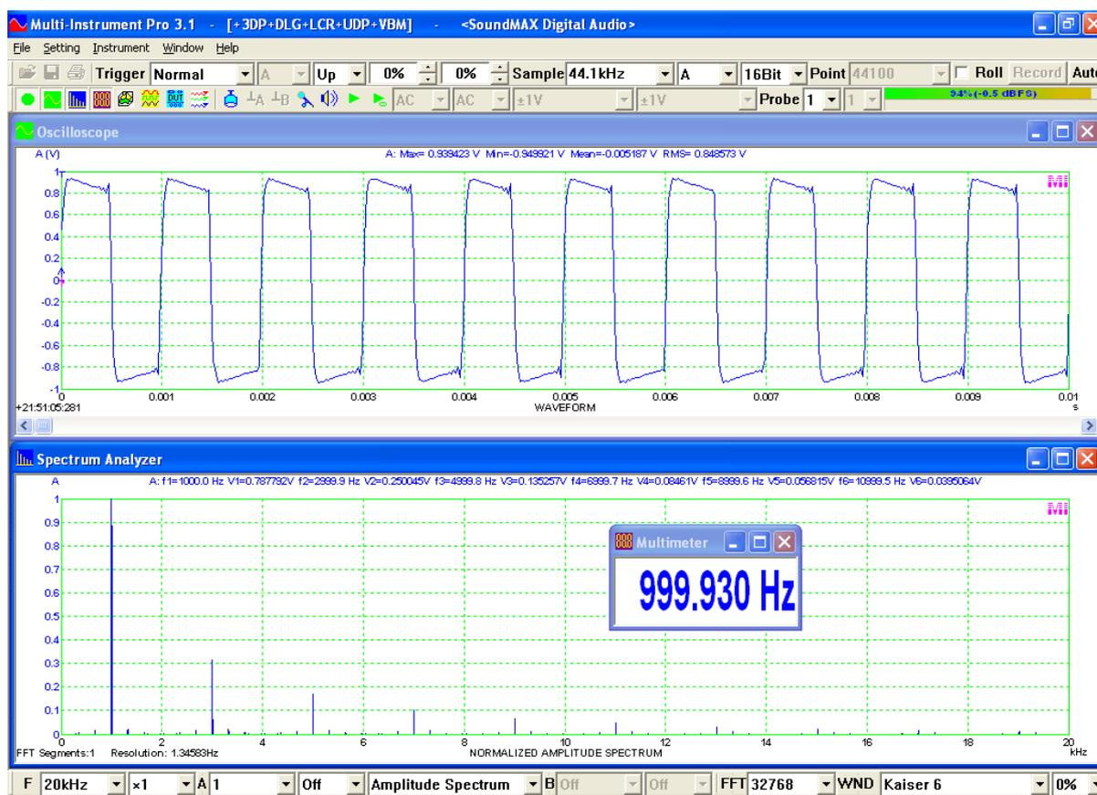
The oscilloscope in the above screenshot shows that the waveform was triggered right at 0V (Trigger Level = 0%) upward (Trigger Edge = Up). The square waveform measured is reasonably good in shape despite that the top and bottom of the waveform is not so flat as the ideal one, which can be attributed to the limited bandwidth and phase distortion of both the output channel of the Pocket PC and the input channel of the laptop.
