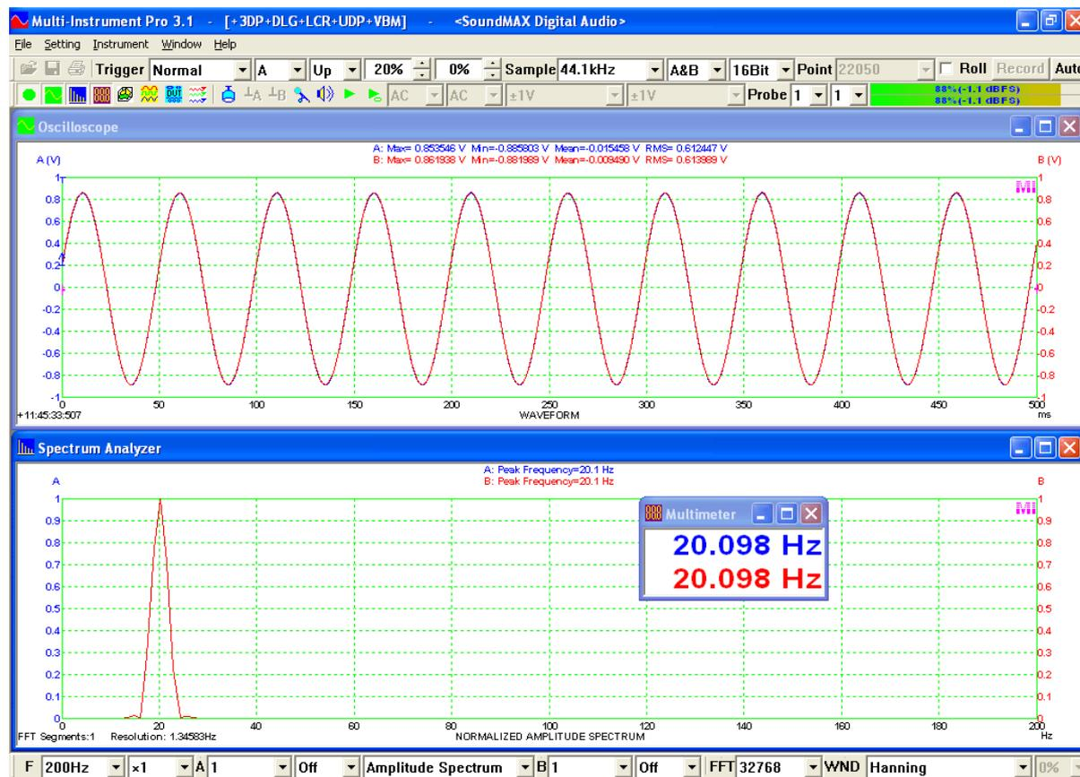
The oscilloscope in the above screenshot shows that the waveform was triggered right at 0.2V (Trigger Level = 20%) upward (Trigger Edge = Up). The stability of the triggered waveform display was excellent and no shaking left and right or up and down was seen.
