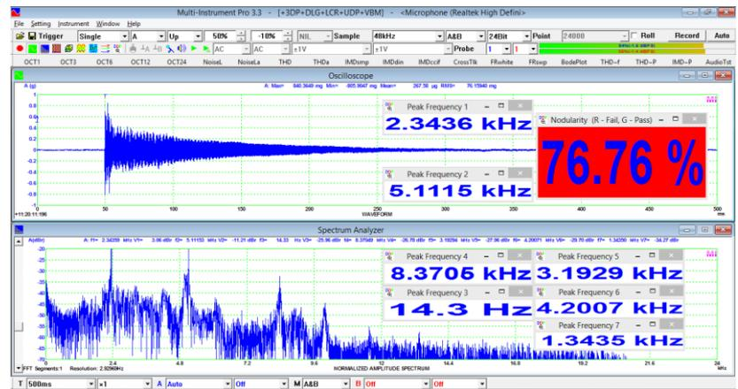
(Impact Test by detecting multiple frequency peaks)
