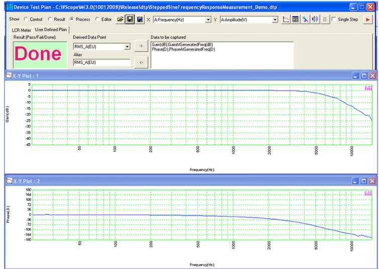
(Gain and Phase Plot using frequency stepped sine)
