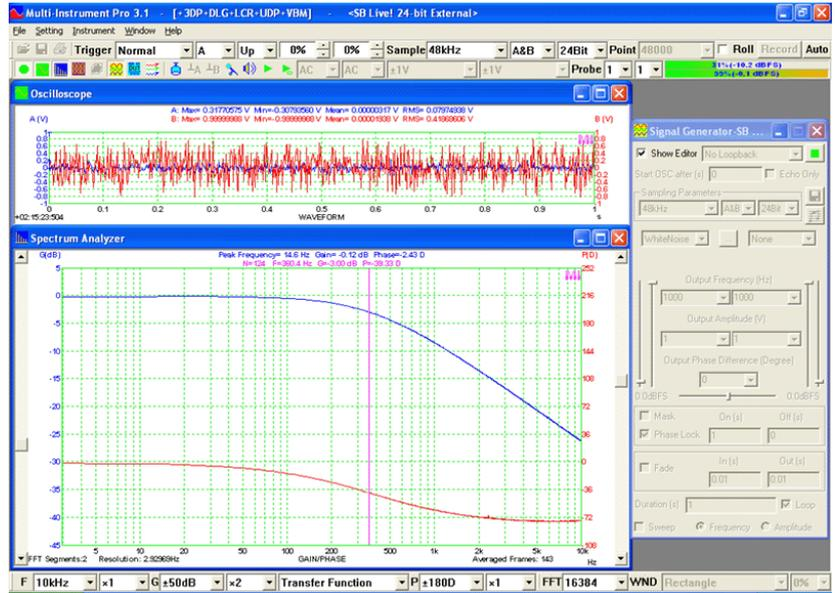
(Measurement of Transfer Function (Bode Plot) using Dual FFT)
