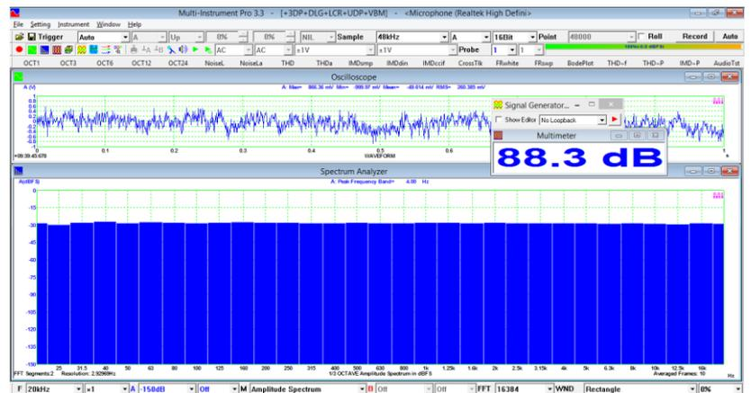
(Frequency Response Measurement using pink noise and octave band analysis)
