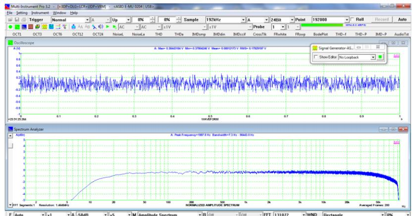
(Frequency Response Measurement using white noise and narrow band spectrum analysis)
